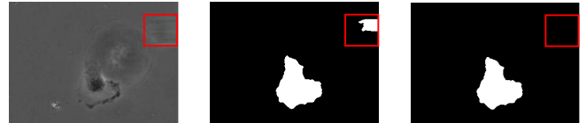
(a) Raw input image. (b) Result of baseline U-net. (c) Result of tiling-based framework.
